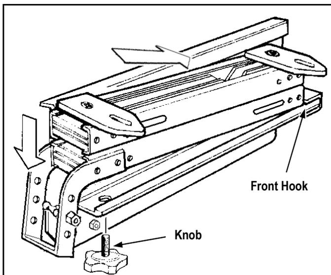
**6 Install the Kick Stands on the Saddles.** Then place them on the Truck Bed. You'll make the final adjustment to the Kick Stands after the Saddle and Clamps have been tightened.
