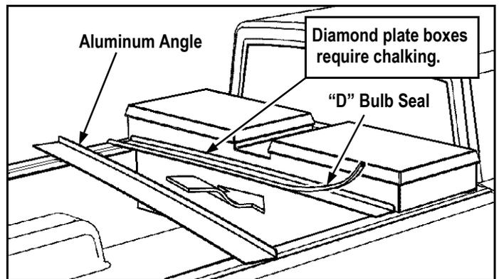
**4 Fitting the Lid.** Have a person get into the truck bed with a flashlight and a tape measure. Place the Lid on to the truck and adjust it so that it fits evenly on both sides and across the tailgate. Once this is done, have the person inside measure the distance between the center of front Lid Mounting Stud and the Tool Box Wall. Measure this distance on both sides. Remove the Lid after the measurements are taken.
