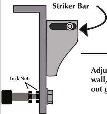
Adjusting the striker bracket is quick and easy. Drop the tailgate, close the lid down, and determine where the center of the latch will need to catch. The striker can easily move vertical and also forward/backwards. This must be done on every installation; Truck beds will vary slightly. Gaylord's suggests monthly inspection of these parts to ensure perfect locking and unlocking for the duration of ownership.
