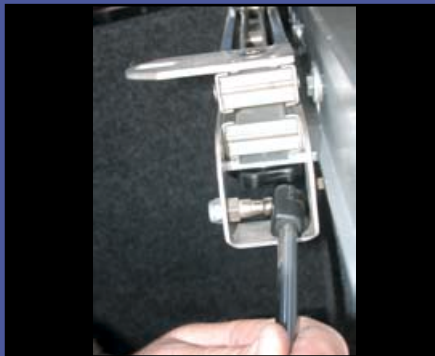
14. The gas struts are then attached to the H-hinge. The lock must be removed and then reattached once the struts are in place.
