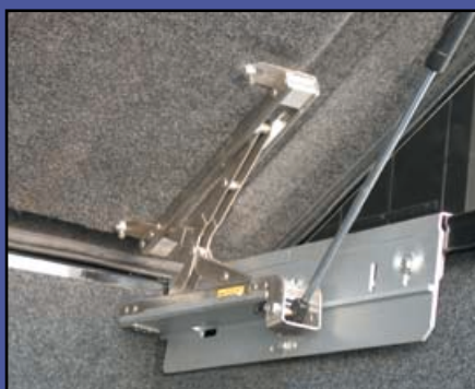
19. You can see how simple the system is and how well it works at distributing the weight of the tonneau across the hinge.
