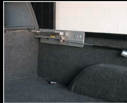
15. The struts are left loose until the tonneau is reinstalled onto the bed.
