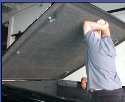
17. With some help the struts are attached to the underside of the tonneau.
