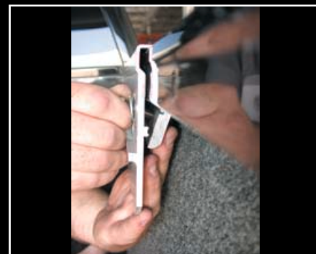
6. A total of three clamps are used to secure the brace to the bed rails. These are mounted loosely so that the brace can be properly adjusted.
