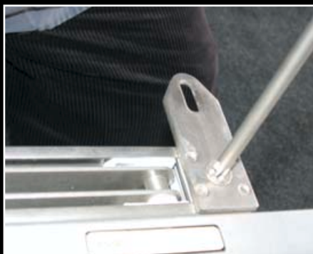
4. Two tonneau brackets attach to the H-hinge and will bolt up to the studs that will protrude from the underside of the tonneau.
