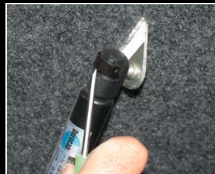
18. Two brackets are already attached to the underside of the tonneau and the struts simply snap on. The locks are then pushed into place to prevent them from popping out.
