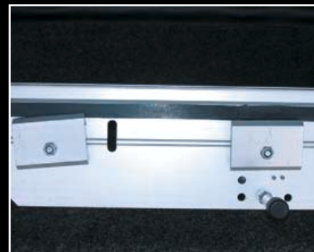
3. The clamps and side brace were attached to the hinge brackets. They will clamp against the underside of the bed rails.
