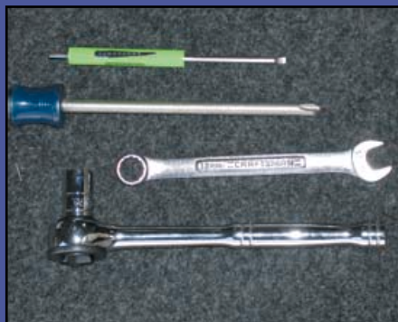
2. Only a few tools are needed to install a tonneau such as this one. We used a 13mm socket and open end wrench, Phillips screwdriver and a small flat-head screwdriver.
