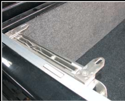
13. This is what the brace and H-hinge looks like when it is properly bolted to the bed rails.
