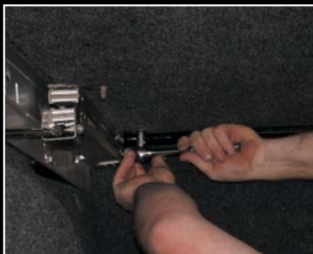
16. With the tonneau back on the bed, it is finally bolted onto the H-hinge from underneath.
